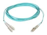
Fiber Optic Patch Cord, OM3, LC to SC duplex, 1.8 mm LSZH & OFNR, 3 m, agua  $\,$
